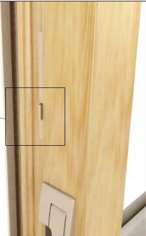
The Ultimate Glider features tabs to help in confirming whether or not your window has locked. If the window has been closed completely and you do not see the tab, the window is locked. In the illustration above, the tab is protruding from the stile which signifies the window is not locked. If your window has not been installed square in the opening, the tabs will indicate that lock adjustment is needed. See your local dealer for help with lock adjustment.
