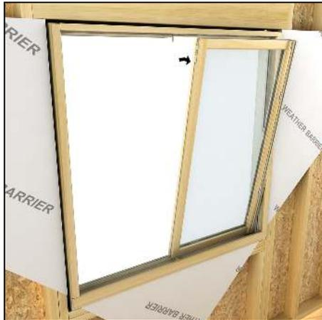
Removing sash for XX configuration
