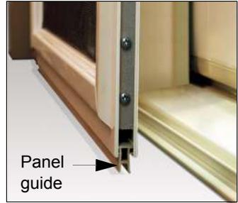
The screen can be adjusted from the interior by loosening or tightening the top roller screw nearest the locking jamb. Adjust the screen so that it is parallel to the locking jamb or casing. An even reveal should be achieved along the entire height of the jamb. If more adjustment is necessary, the other roller adjustment screw can be used but the screen panel will need to be removed for access.
